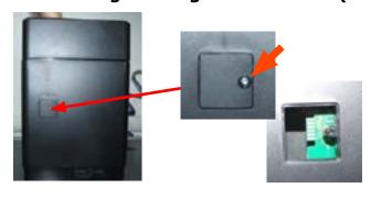
Loosen the screw for remove the cover.
