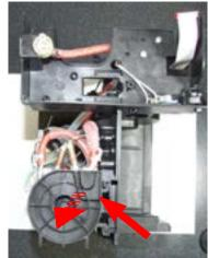
Unscrew the screw shown at unthread the support boiler
