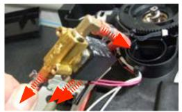
Disconnect all electrical and water circuit connections
