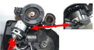
Raise the coffee grinder and remove the connections.
