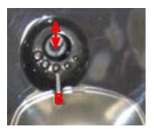
To adjust grinding further, the engineer can work directly on the coffee grinder by pressing and turning the ring nut (C) shown. (clockwise + to increase the particle size of the coffee and anticlockwise - to decrease it).
