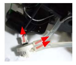
Lift the flow meter out of the casing assembly and remove the electrical and water circuit connections.
