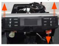
Remove the board support assembly and disconnect the electric connection
