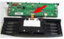
Disconnect the electrical connections.
