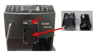
Unscrew the screws shown and remove the dispenser
