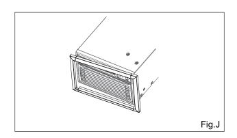
Note:Be sure to route the cord through the trim frame before placing the trim frame on the unit.
